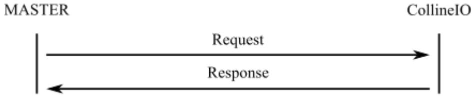
The commands from the master can use the RS-485 or RS-232 port. Commands are Modbus RTU compatible. Optionally master systems can be RaspberryPi (student or amateur) or any other CPU format size compatible (for example, i.MX6UL Module from Digi) for industrial environments.
