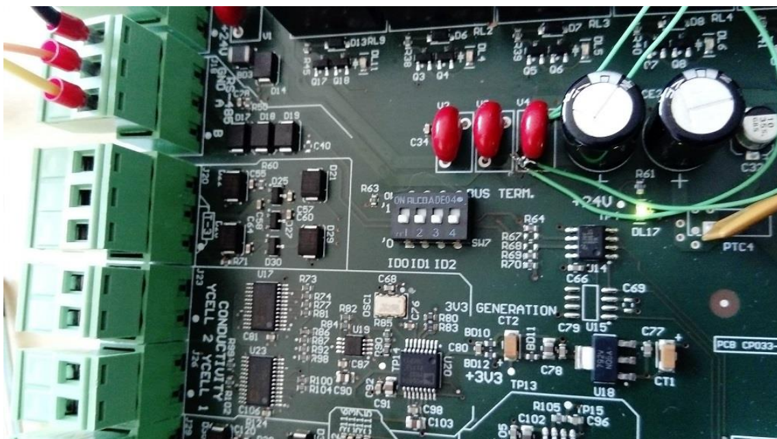
Figure 3: SW7 Microswitch for board ID and RS484 bus termination resistor
